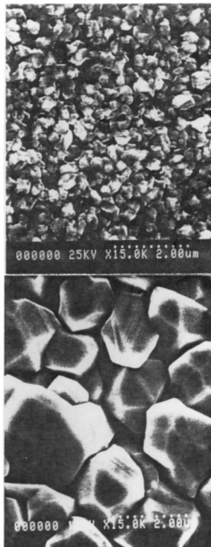
Figure 3. (a, top) Scanning electron micrograph of small-grained film deposited at 200 °C from (hfac)CuPMe 3 . (b, bottom) SEM of large-grained film deposited at 400 °C from (hfac)CuPMe 3 .
